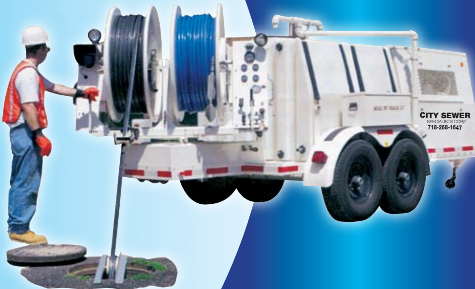
High pressure water jetting from 12" through 38" diameter lines
